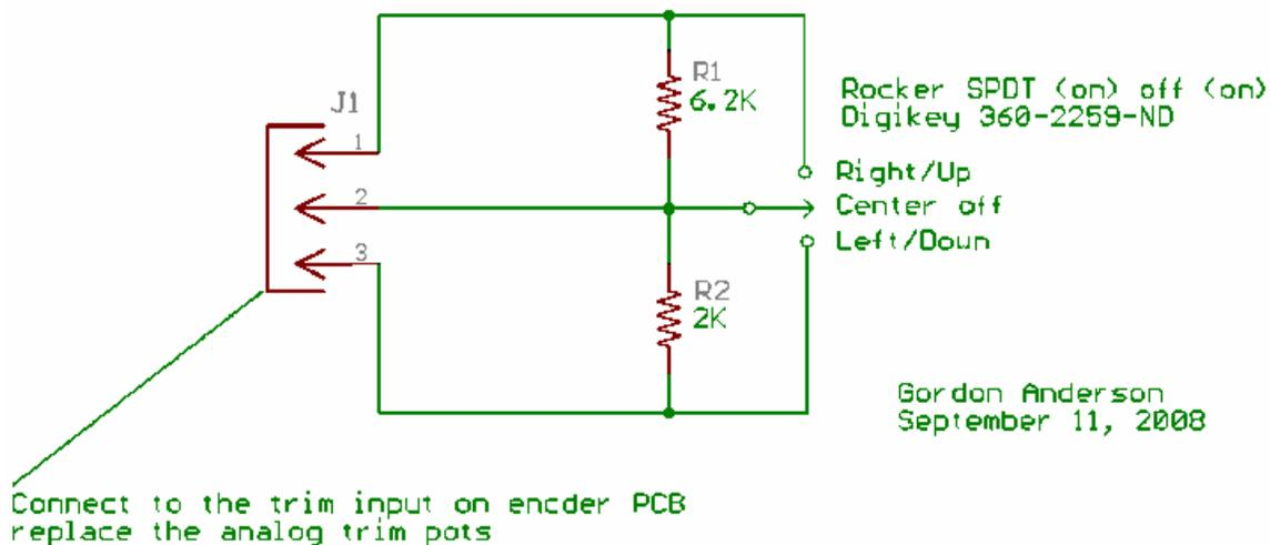
The circuit configuration for the digital trim switches assumes you are using standard analog trim configuration with the battery voltage being applied to the trim pots and the trim pot series resistors set at 4.7K (RN3 on the rev 4.0 Encoder hardware). If you use 5 volt regulated power on your trims and the series resistor values have been set at or below 1K you can use two 4.7K resistors for R1 and R2 in the circuit shown above.
