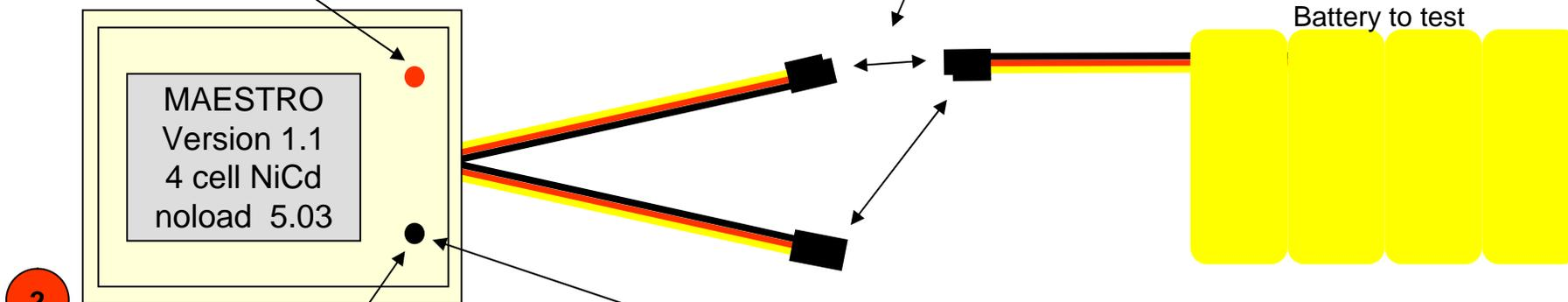
2 Momentarily press this button to test the voltage under load.
