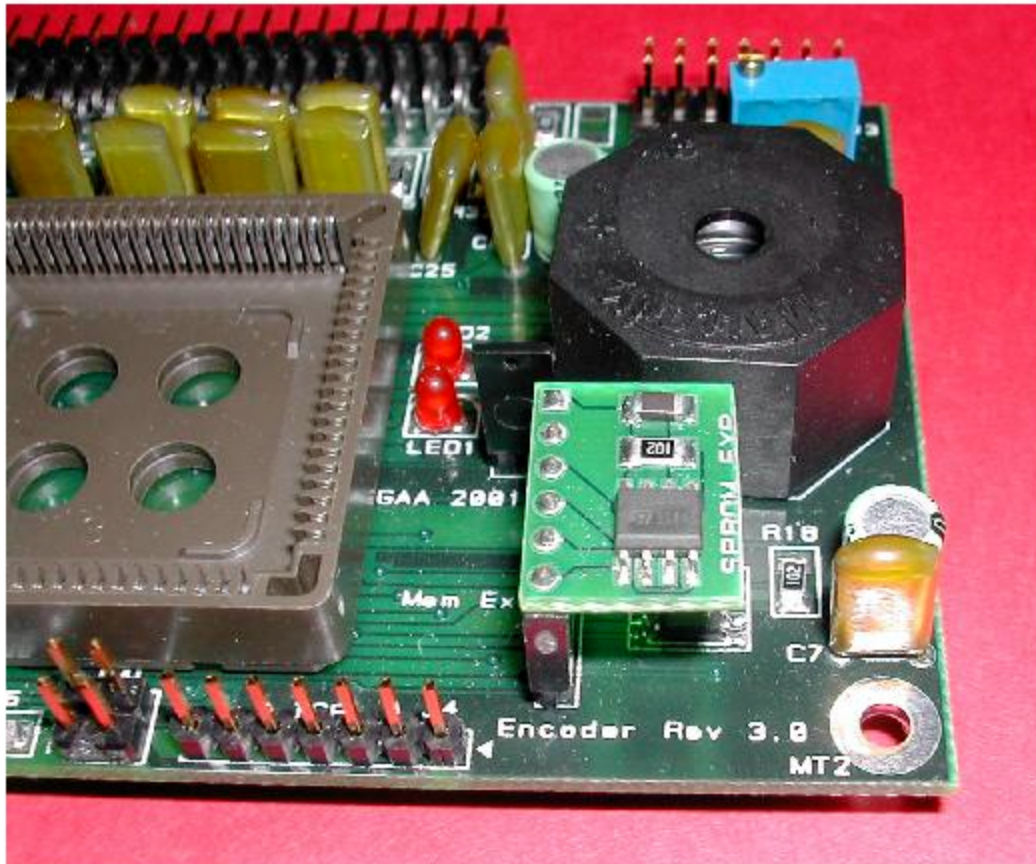
Expansion module installed in Encoder
