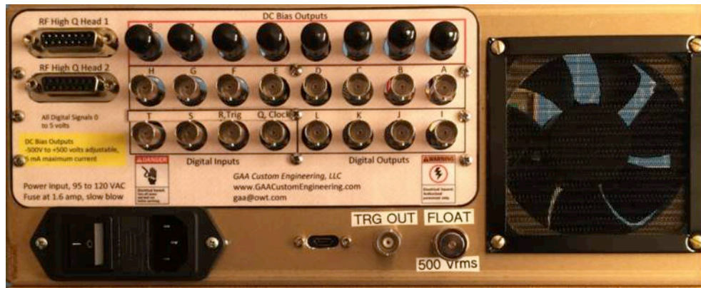
MIPS rear panel connections. Note the black cap-plugs installed of DC bias outputs as a safety precaution.
